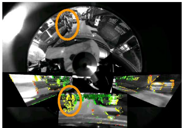
Fig. 5. Stereo computation result with 3 views of a traffic scene. Note the slight overlap of the 3 views.
