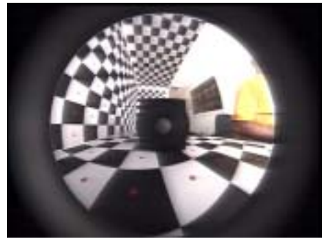
Figure 7: Real image taken by our catadioptric system with a hyperbolic mirror.
