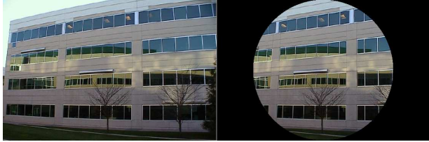
Figure 9: Radial correction result for the Hitachi video camera. Left: input image; Right: output result. (only central-part is showed.)
